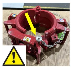
**Figure 1:** Safety Lock Pin installed incorrectly in the latch before the elevator is latched
