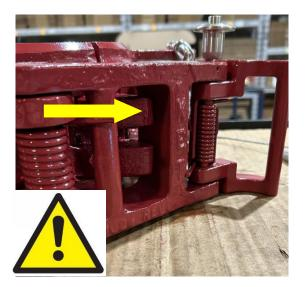
**Figure 3**: Shows the "Partial Latch" that occurs when the safety latch lock pin is used incorrectly
