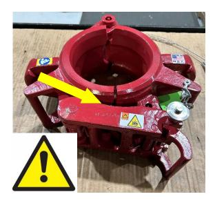
**Figure 2**: Elevator latched incorrectly with the safety lock pin installed in the latch
